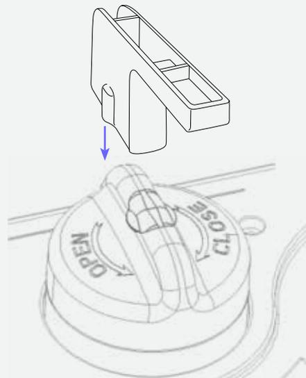
Remove the new MAXI filter cartridge from its packaging and insert it. Then turn firmly clockwise to install.
