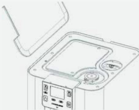
You will see the white top of the MAXI filter cartridge towards the back of your BIBO with a handle protruding from it. Turn the handle firmly anti-clockwise until the filter cartridge releases, then pull it up and out of the BIBO.
