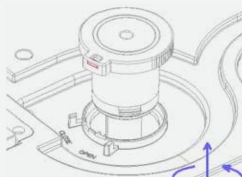
Remove the replacement UV lamp from its packaging and insert it carefully. Then rotate it clockwise to the "CLOSE" position, it will click and lock.
