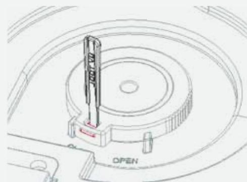
You will see the white cap of the UV filter lamp towards the front of your BIBO. Locate the small, white plastic key supplied with your new UV lamp. Put the key in the slot as indicated below, release the latch and rotate the UV lamp anti-clockwise to the "OPEN" position. Pull the UV lamp up and out of the BIBO.
